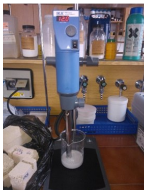
Fig. 1: Homogenizer ULTRA-TURRAX T25, IKA during homogenization of the mixture with MFC.
