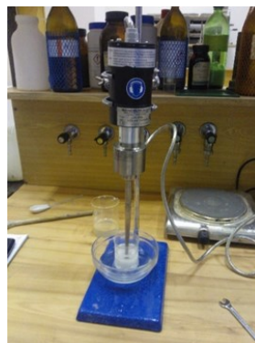
Fig. 2: Ultrasonic homogenizer Bandelin SONOPULS during homogenization of the mixture with NFC.
