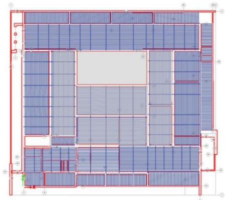
Fig.6.d. Modelled ground floor top view in ETABS
