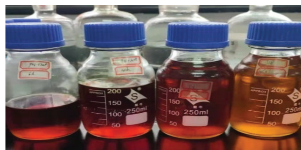
Figure 3. Oil samples of a certain domestic aviation lubricating oil oxidized for 8h, 4h, 1h and 0.5h at 200°C
