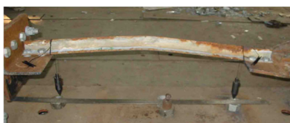
Figure 4. Axial compression member failure mode
