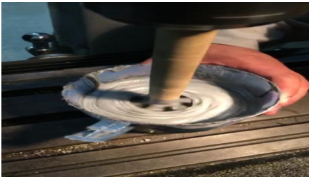
Fig. 1: Material Mixing through Shear Mixer
