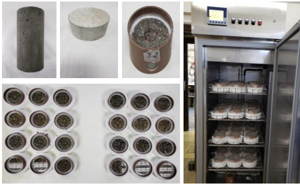
Fig. 3. Concrete specimen disks prepared for freeze-thaw and mass scaling tests.
