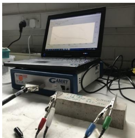
Fig. 3: EIS potentiostat test set up (Gamry device)
