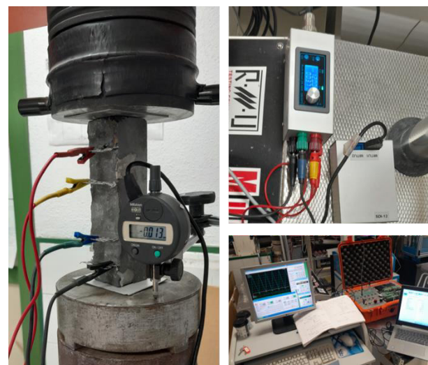
Fig. 5. PZR test setup for 40 x 40 x 160 mm specimen.
