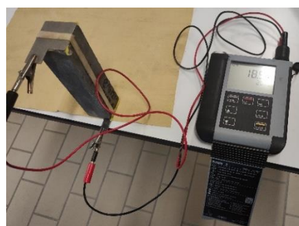
Fig. 3. Set up for electrical conductance measurements.
