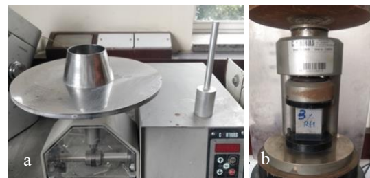
Fig. 2. a) Flow-table set-up b) Compressive strength test
