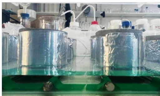
Fig. 4. Specimens sealed laterally with aluminium foil and partially submerged in water for capillary absorption.
