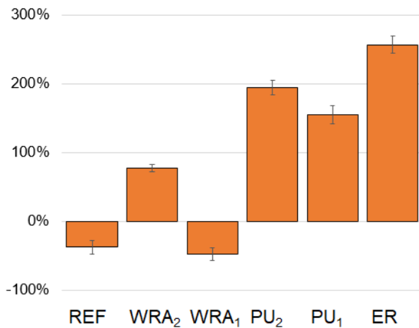
Figure 5. Load regain index (LRI) of each series. Error bars indicate standard deviation of three samples.
