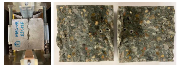
Fig. 8. Splitting the cube specimens to count the amount of broken capsules in a certain crack plane (note: the darkest concrete surface is the area covered by WRA)
