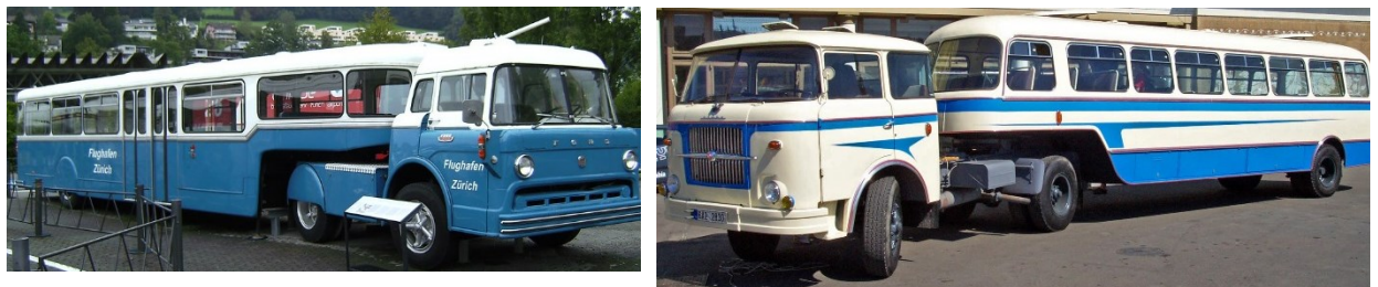
Fig. 1. Airport buses of the 50s and 60s of the last century: a - a Ford tractor unit with a passenger semi-trailer used at the Zurich airport; b - a Skoda truck with a semi-trailer based on a Skoda bus.
