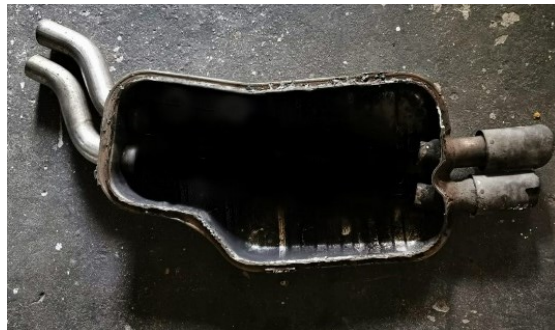
Fig. 5. The design of the silencer in the fourth variant.
