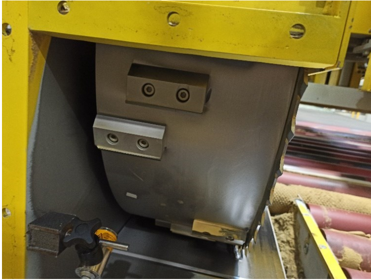
Fig. 3. View of the mating surface of the drum saw with mounted knives.
