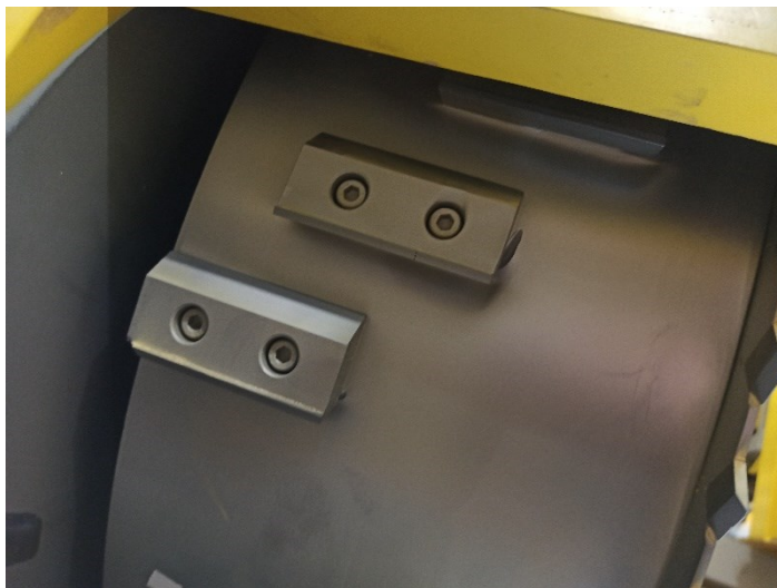
Fig. 4. View of drum knives.
