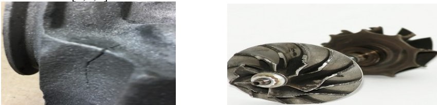
Fig. 2. Fracture of the outer part of the housing.
