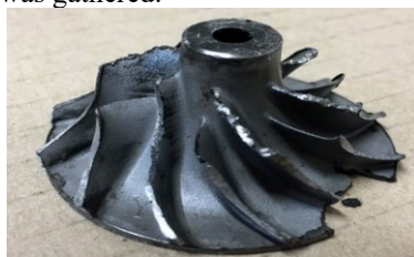
Fig.10. Cracked compression wheel.
