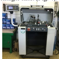
Fig.5. Rotor balancing machine.
