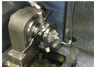
Fig.7. Balancing the turbocharger shaft. Fig. 8. Balancing the core of the turbocharger.
