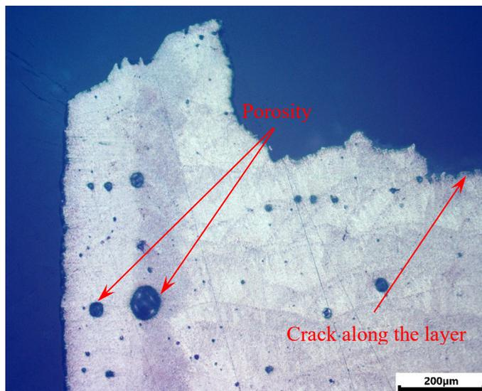
**Fig. 1.** Microstructure of AISi10Mg aluminum alloy produced by SLM technology: a) as-built state on a surface parallel to the build direction, b) after a static tensile test on a surface perpendicular to the build direction [own research]
