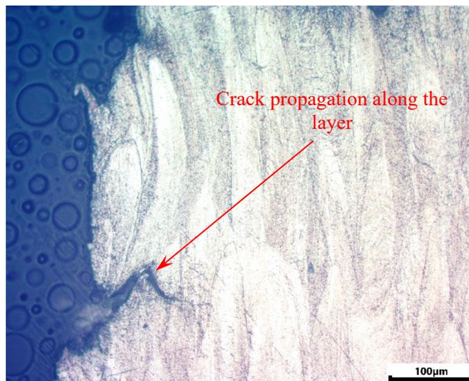
**Fig. 2.** Microstructure of L316 stainless steel produced by SLM technology: a) as-build state on a surface parallel to the build direction, b) after a static tensile test on a surface perpendicular to the build direction [own research]
