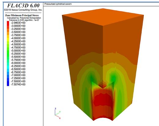
**Fig. 8.** Distribution of tensions for a pressure of the cavern of P=2.9MPa.
