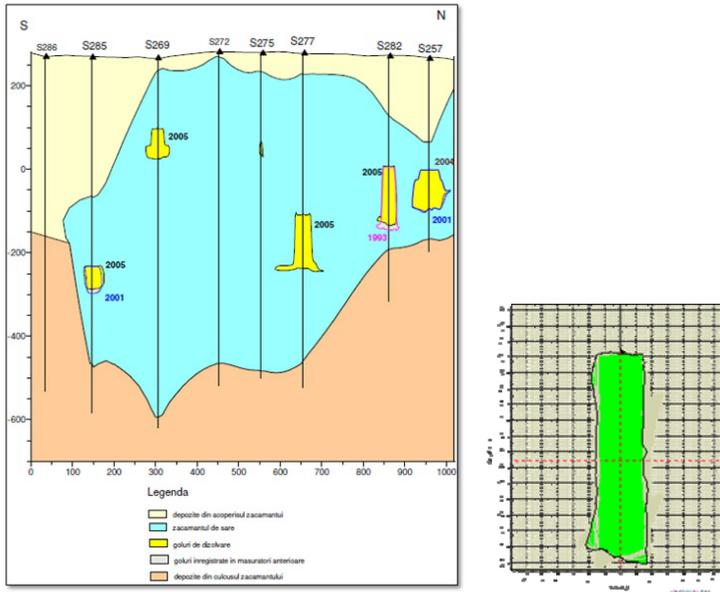
**Fig. 5.** Vertical sections through salt caverns from the perimeter of the Gura Slamic Tg.Ocna.
