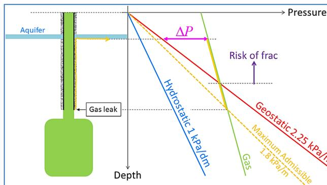
Fig. 3. The pressure gradient depends on the depth of the deposit.
