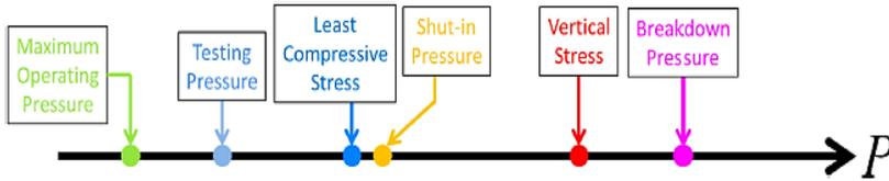
**Fig. 4.** Selection of maximum operating pressure in a salt cave.
