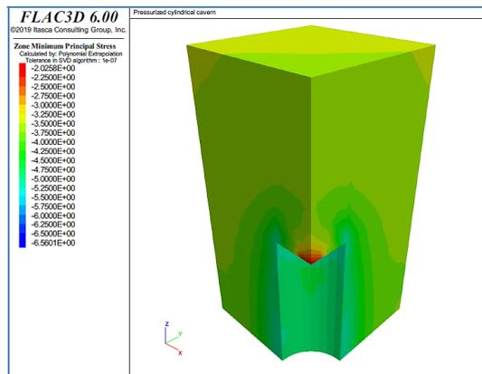
**Fig. 9.** Distribution of tensions for a pressure of the cavern of P=0 MPa.
