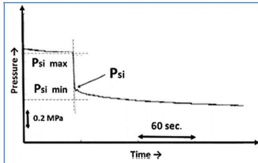
Fig. 2. Schematic procedure for FRAC test [4].
