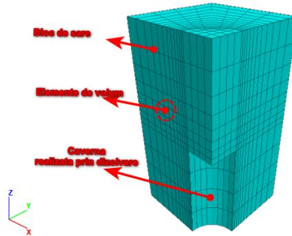
**Fig. 6.** 3D model and discretization with volume elements.
