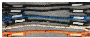
Fig. 5. Samples exposed to conditioning A and flame
