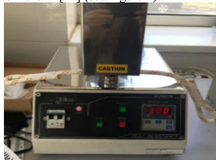
Fig. 2. Apparatus for testing contact heat resistance
