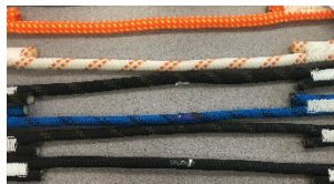
Fig. 6. Samples exposed to A conditioning and contact heat
