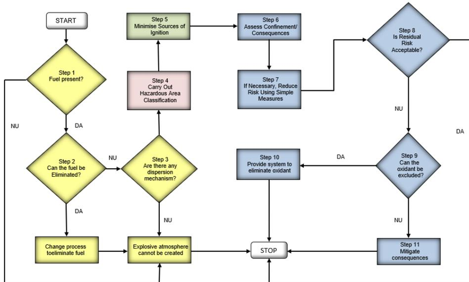
**Fig. 6.** The explosion risk logic diagram
