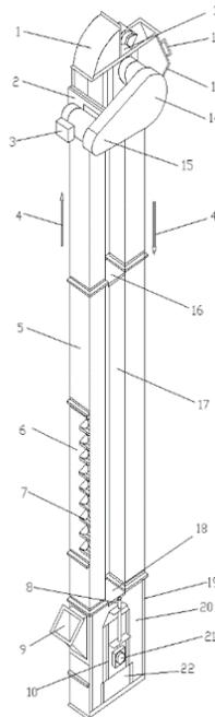
**Fig.3.** – Two-legged bucket elevator - components
