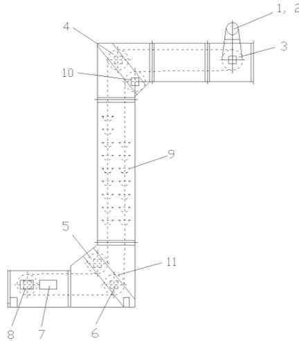
**Fig.5.** – Z-type bucket elevator - components
