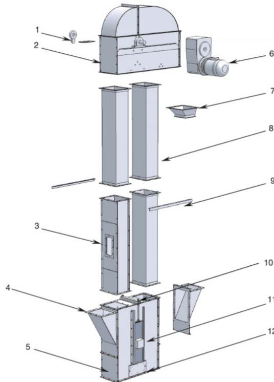
**Fig.2.** – Bucket elevator - components
