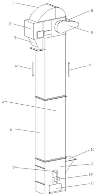
**Fig.4.** – Single leg bucket elevator - components
