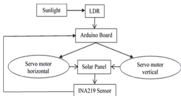
**Fig. 1.** Block diagram of Arduino-based dual axis solar tracking system prototype.
