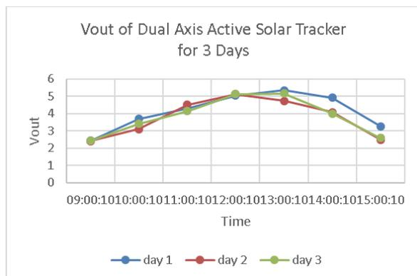
**Fig. 4.** The output voltage of the dual axis active solar tracker for three consecutive days.
