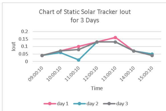
**Fig. 8.** The output current of the dual axis static solar tracker for three consecutive days
