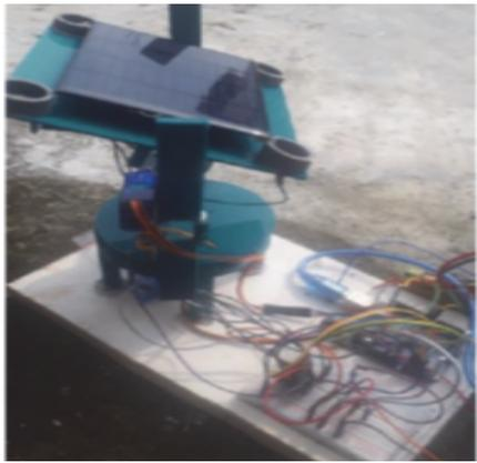
**Fig. 3.** Arduino-based dual axis solar tracking system prototype
