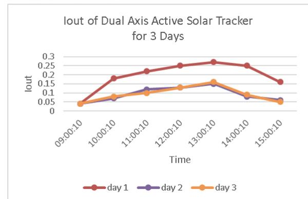
**Fig. 5.** The output current of the dual axis active solar tracker for three consecutive days.
