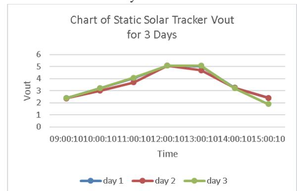
**Fig. 7.** The output voltage of the dual axis static solar tracker for three consecutive days
