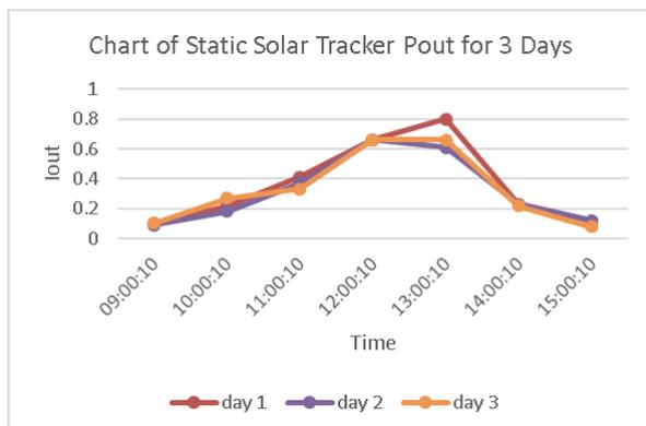
**Fig. 9.** The output power of the dual axis static solar tracker for three consecutive days
