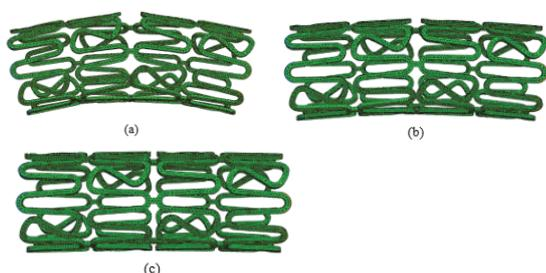
**Fig. 6.** Crimped stent simulation results curvature index changes: (a). 50 $\mu\text{m}$ , (b). 60 $\mu\text{m}$ , (c). 70 $\mu\text{m}$
