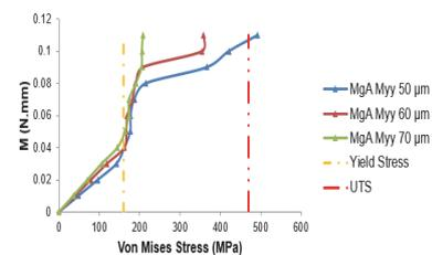
**Fig. 5.** 5a. Simulation results of curvature index with crimped stent using Magnesium Alloy AZ31 with
