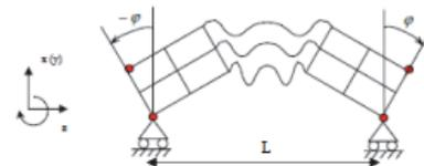
**Fig. 4.** Angle change in stent due to bending moment
