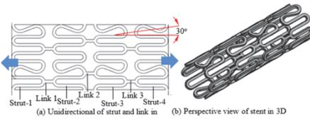
**Fig. 1.** Stent Design S<sub>S</sub>: (a). 2D perspective. (b) 3D perspective.
