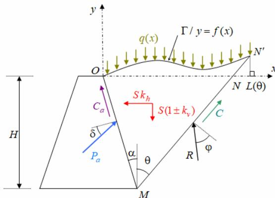
**Fig. 1.** Retaining wall and backfill soil wedge system with representation of all the acting forces.
