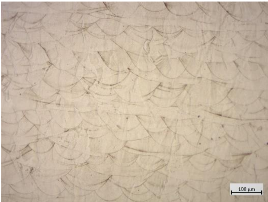
Fig. 4. Optical micrograph of a cross section of an as-built specimen perpendicular to the Z-axis (in the XY plane) at 10x magnification
