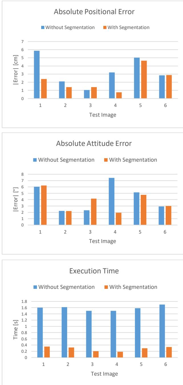
**Fig. 5.** The execution time (bottom), the attitude error (middle) and the positional error (top) of the different approaches.
