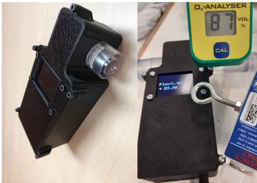
Fig. 13. Rapidly created production line Flow / Pressure / Oxygen Tester
