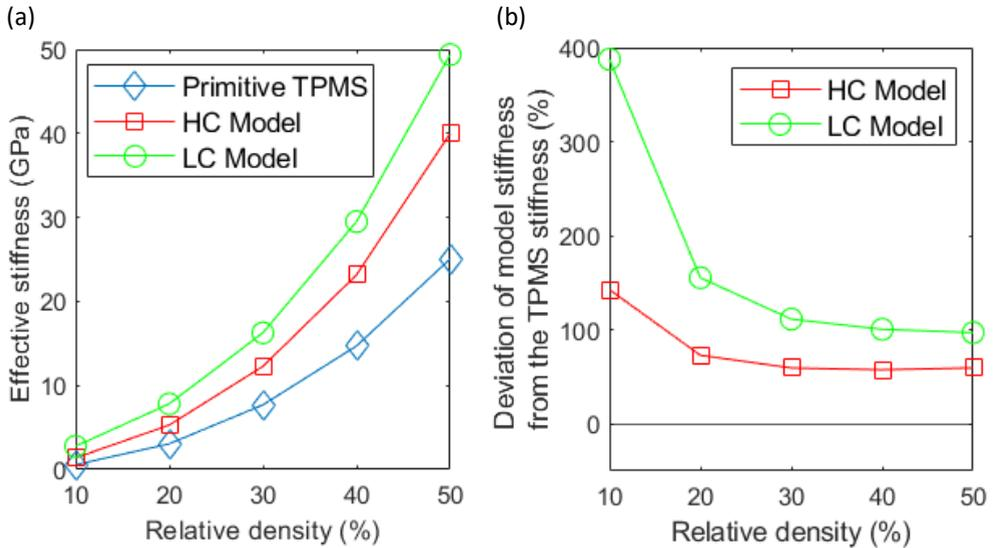
**Figure 3. (a) Effective stiffness vs relative density, (b) Deviation of model stiffness from the TPMS stiffness.**
