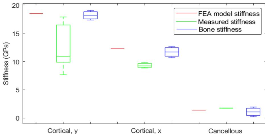
**Figure 8. Comparison between FEA model-, experimentally measured-, and bone stiffnesses.**
