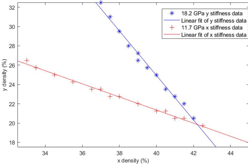
**Figure 5. Lines of constant stiffness derived from the intersection of the planes in Figure 4.**
