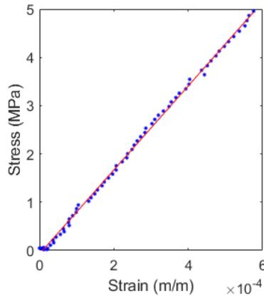
**Figure 7. Stress vs strain graph of a single test for a cortical-based structure with strain measured in the y direction.**
