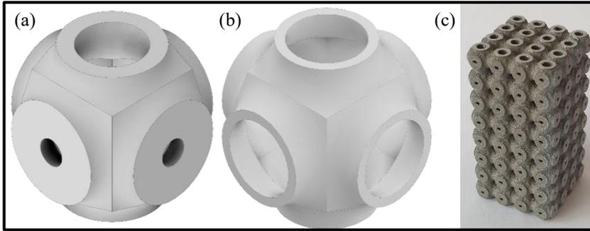
**Figure 6. (a) Final cortical model, (b) final cancellous model, and (c) titanium cortical structure**
