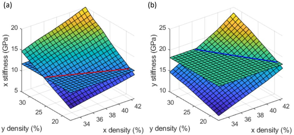
**Figure 4. (a) Stiffness in x direction as a function of varying relative density in the x and y directions and (b) stiffness in y direction as a function of varying density in the x and y directions.**
