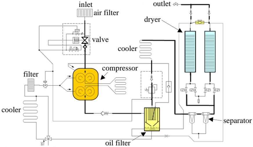
Fig. 1. Compressor circuit
