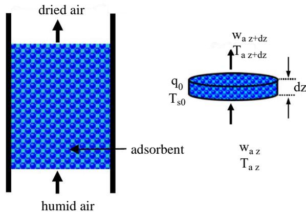
**Fig. 3.** Discretization of adsorber column [7]
