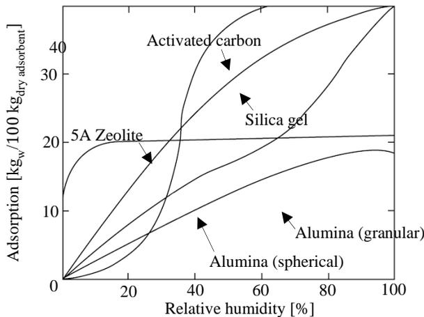
**Fig. 5.** Adsorption isotherms of water vapour from atmospheric air [8]
