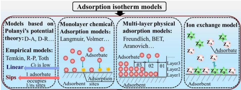
Fig. 2. Adsorption isotherm models [6]
