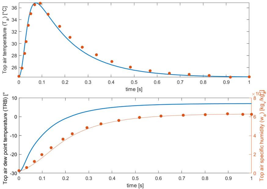
**Fig. 6.** Comparison of the adsorption process using silica gel
