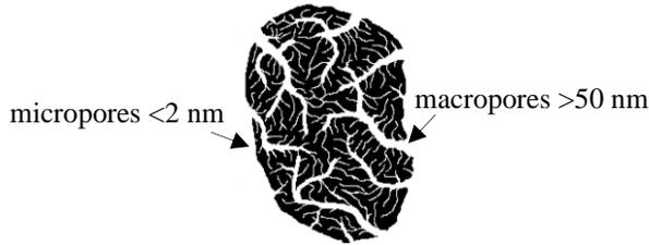
**Fig. 4.** Types of pore in adsorbent [5]
