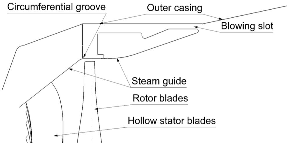
**Fig. 1** Steam turbine cross section in the area of last stage tip
