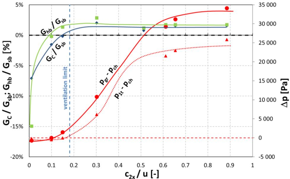
Fig. 4 Courses of pressure differences and relative flows depending on  $c_{2x} / u$  for the monitored turbine
