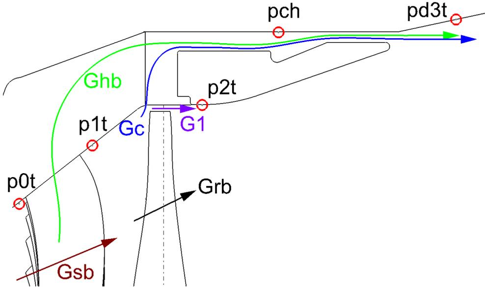
**Fig. 2** Measured pressured and calculated mass flows
