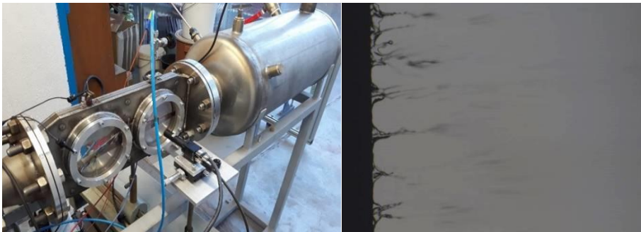
Fig. 1. The wind tunnel and the water film breakup on the trailing edge of the blade.
