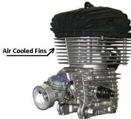
**Fig. 1.** Air cooling system [3]
