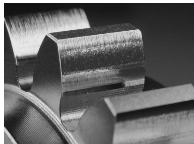
Fig. 1. Typical scratches on the addendum and dedendum of a tooth flank due to slow speed wear [6].
