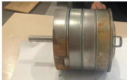
a) rotor part of the pump
