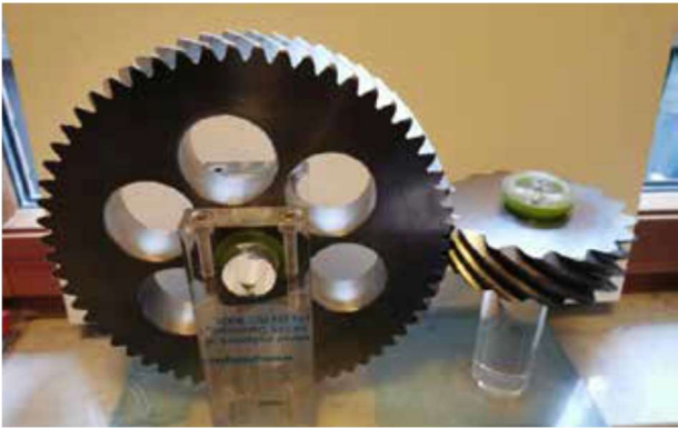
Fig. 17. Working model of the crossed helical S-gear drive
