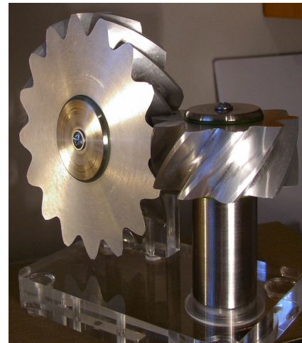
Fig. 15. Model of a crossed helical gear with a progressively curved path of contact, \beta = 45^\circ
