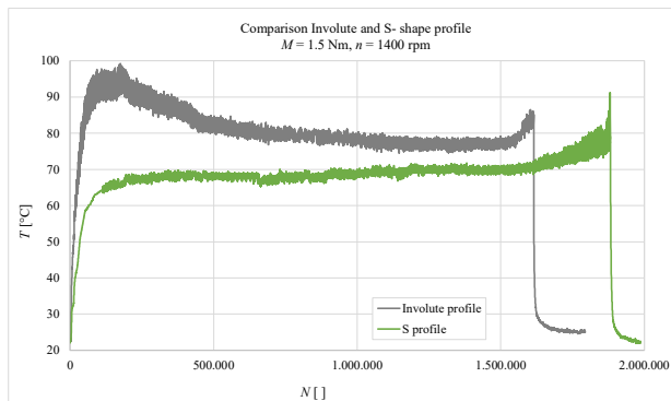
Fig. 14. Comparison of E- and S-gearing with the steel pinion and POM wheel at M = 1.5 \text{ Nm} and n = 1400 \text{ min}^{-1} a.) temperature spot in the meshing area E (left) and S (right) gear. b.) temperature-time profiles (S – green, E – grey) [15]
