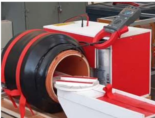
Fig. 1. The device generates a magnetic field to align fibres in fresh concrete.
