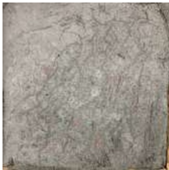
Photo3-1 Initial crack test results for copper fiber
