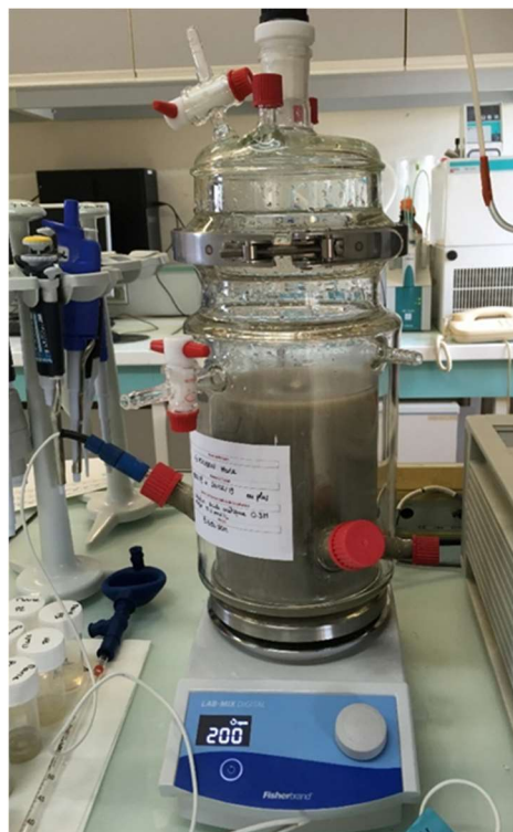
Figure 1. Experimental device for the study of the degradation of OPC paste powder by an ammonium nitrate solution
