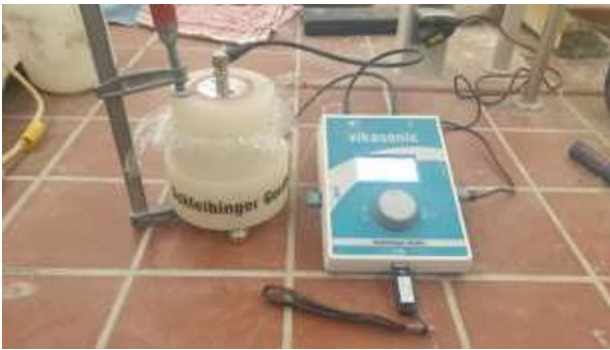
Figure 2 : Experimental setup of the Vikasonic ultrasonic device.
