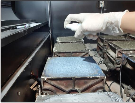
Fig. 1. Spraying of curing compound.
