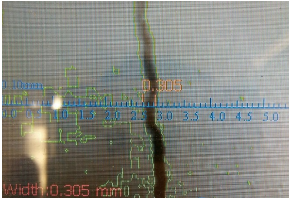
Fig. 6. Initial crack created by tensile split test.
