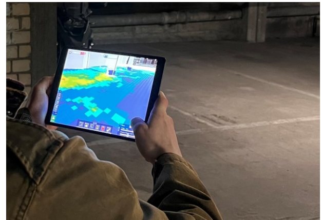
Fig. 12. Application of enriched BIM-models in situ via augmented reality (© Domenic Graffi)
