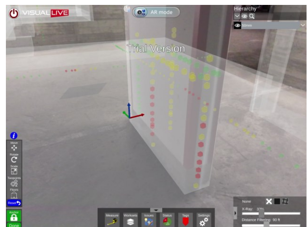
Fig. 14. AR-Visualisation of concrete cover (red < 15 mm, yellow < 30 mm, green \geq 30 mm) in VisualLife
