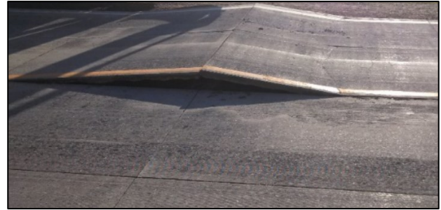
Fig. 7. Buckling in a COA-U overlay [10].
