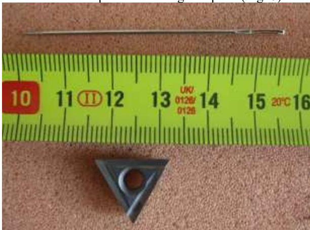
Fig. 4. Scratch test tools used during pilot experiments.
