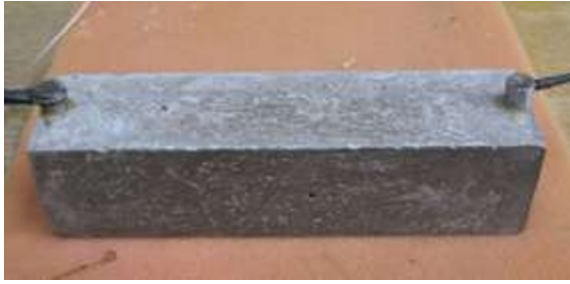
Fig. 3. Location of piezoelectric sensors during testing.
