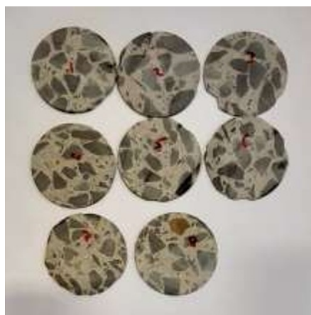
Figure 4: Bulk diffusion test: (a) concrete specimen; (b) sliced specimen
