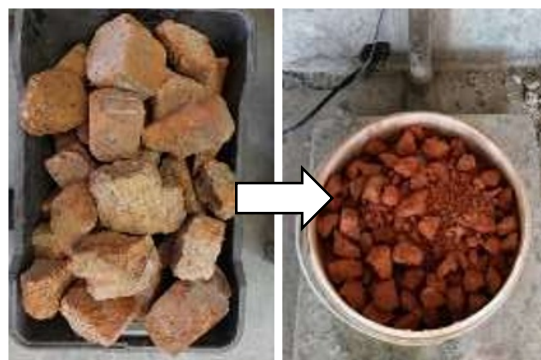
Fig. 2: “Cleaned” clay masonry bricks crushed into smaller aggregate fractions.
