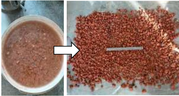
Fig. 4 Crushed CMRB soaked in water and subsequently laid out to dry.
