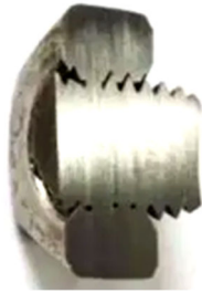
Fig.2 Picture showing the thread locking of austenitic stainless steel bolt
