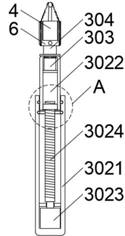
Fig. 3 Structural diagram of telescopic rocker arm
