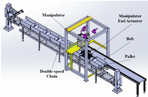
**Fig.1** System of palletizing
