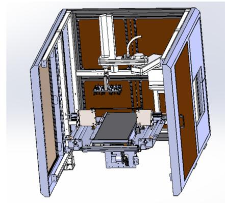
**Fig.2** Rigid palletizing system
