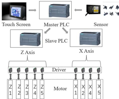
**Fig.4** Hardware structure of control system
