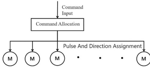
**Fig.3** Schematic diagram of master control
