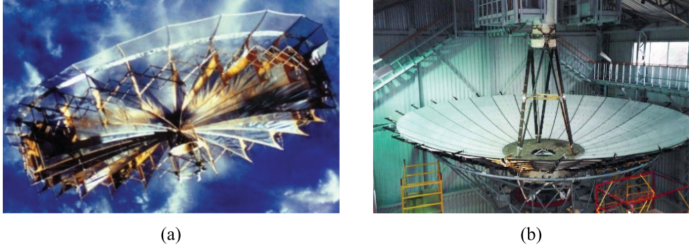
Figure 1. Large-sized transformable space antennas: (a) umbrella-type antenna reflector with a diameter of 12 m; (b) petal-type antenna with a diameter of 10 m
