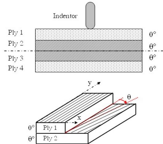
**Fig. 1.** Hybrid composite laminate having four plies and the stacking sequence  $[0/\theta]_s$  where  $\theta$  is the orientation angle.
