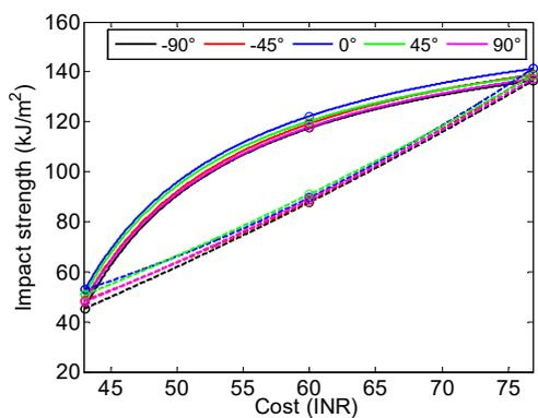
**Fig. 3.** Curves giving impact strength versus cost for the stacking sequences  $[\text{Carbon-Ramie}]_s$  and  $[\text{Ramie-Carbon}]_s$ .
