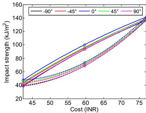
**Fig. 2.** Curves giving impact strength versus cost for the stacking sequences  $[\text{Carbon-Hemp}]_s$  and  $[\text{Hemp-Carbon}]_s$ .
