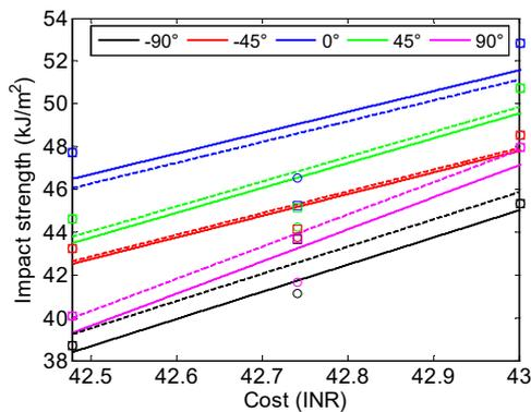
**Fig. 4.** Curves giving impact strength versus cost for the stacking sequences  $[\text{Hemp-Ramie}]_s$  and  $[\text{Ramie-Hemp}]_s$ .
